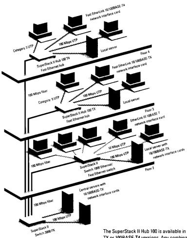
The SuperStack II Hub 100 is available in 100BASE-TX or 100BASE-T4 versions. Any combination of TX and T4 hubs can be stacked and managed together to simply support any type of UTP cable. 100BASE-TX supports Category 5 UTP cable while 100BASE-T4 uniquely supports 100 Mbps on Category 3 or 4 UTP. The 100BASE-FX transceiver module can be used with either hub to provide fiber backbone connections.
